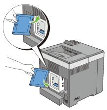
7 Close the control board cover and turn the screw clockwise.
